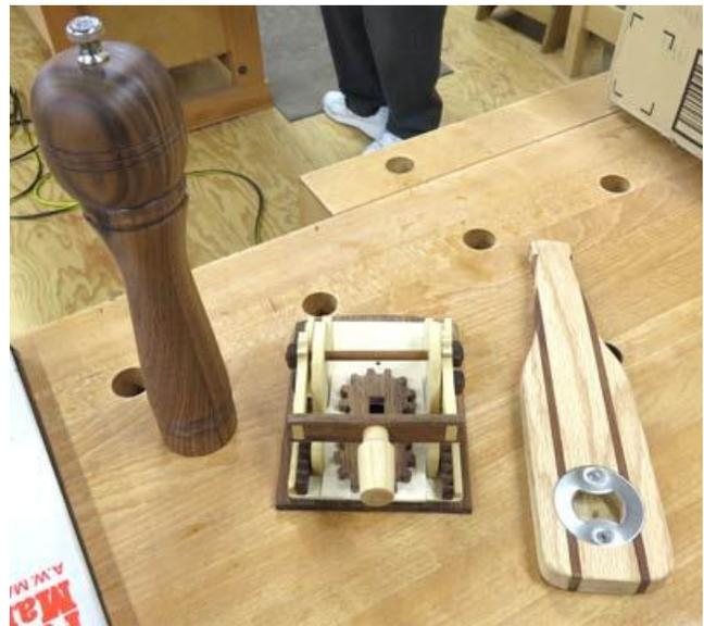
On the right is another useful gadget – a wooden bottle opener in the shape of a beer bottle, made by laminating strips of hardwood like one would for a side grain cutting board. He noted that the metal opener hardware was purchased from **Rockler**. Great projects, **Tom**! Thanks for sharing them with us.
